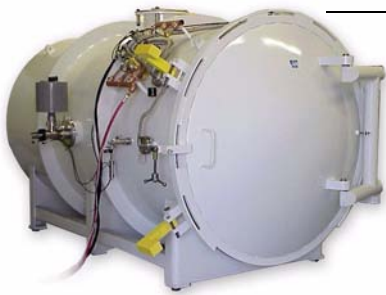
Leak test chamber built for the helium leak testing of large circuit breakers.
