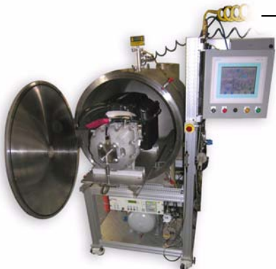
Custom leak test chamber with compressor and slideout
