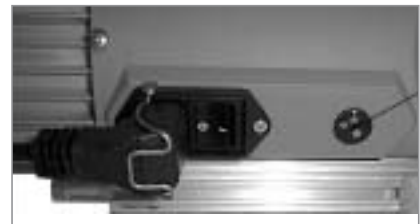
AMD1 power connection
