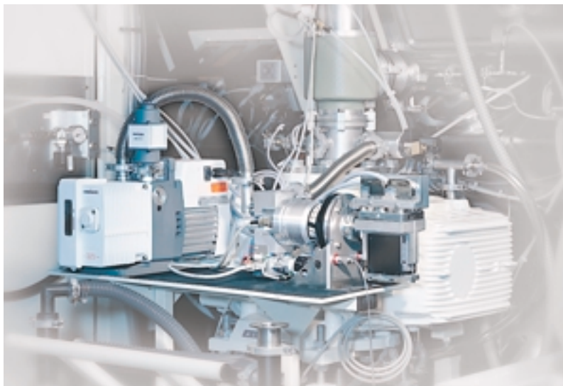
Leak detection system
